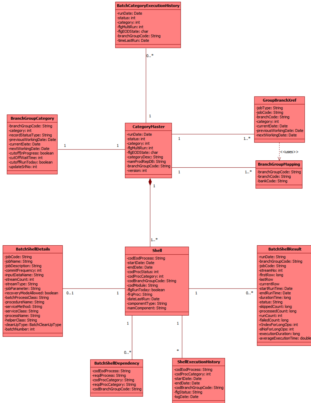
Figure 8–2 Batch Framework Architecture - Static View
